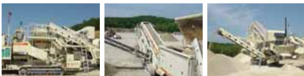
Capital Quarries' Lokotrack system includes an LT110 jaw crusher, an LT1213 impact crusher, an LT300HP cone crusher and three ST620 mobile screens.
